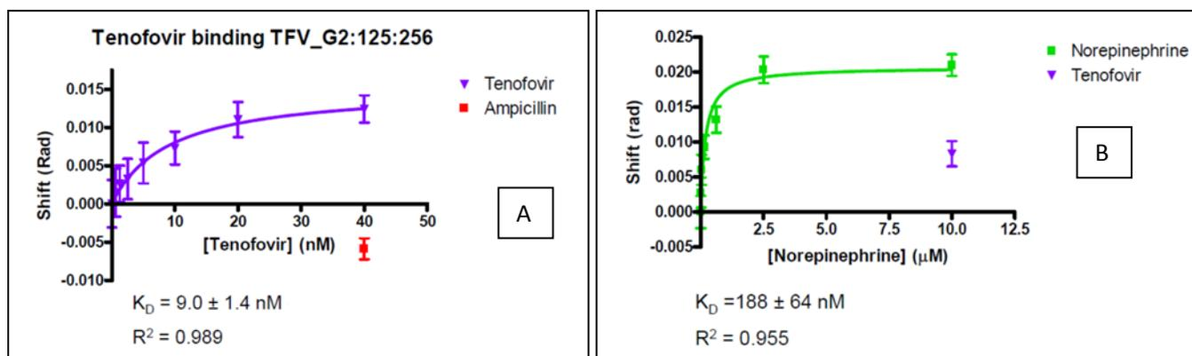
Figure 1. Examples of aptamer:small-molecule binding studies using backscattering interferometry (BSI). (A) A tenofovir specific aptamer is shown to have 9 nM binding and does not bind the small molecule ampicillin (B) An aptamer selected to norepinephrine has a  $K_D$  of 188 nM and shows some degree of cross-reactivity with the small molecule drug, tenofovir.
