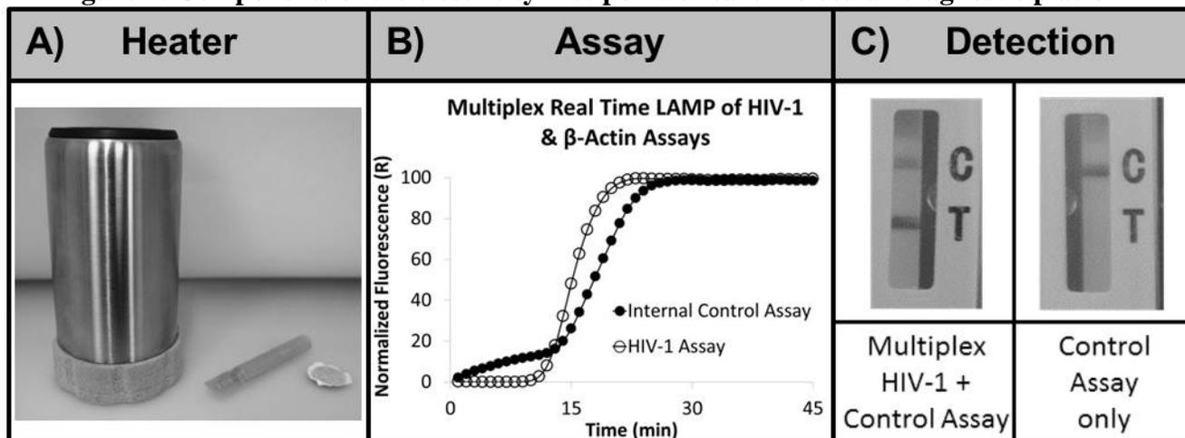
(a) Heater device design, pre-filled saline tube and fuel pouch required for a single run; (b) real time LAMP amplification plots for HIV-1 (○) and beta-actin (●); and (c) NALF cassette with dual amplicon capture lines (Test [T] and Control [C]). The image on the left shows multiplex HIV-1 (T) and beta-actin control (C) detection and on the right, the beta-actin control (C) detection only.
