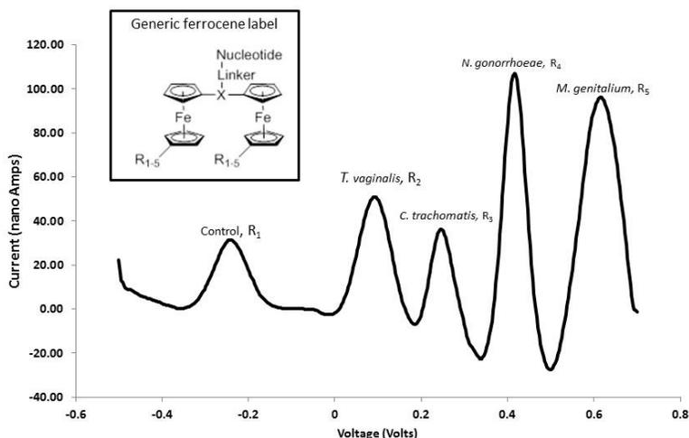
Five-multiplex electrochemical detection of four STI targets plus control from a single sample
