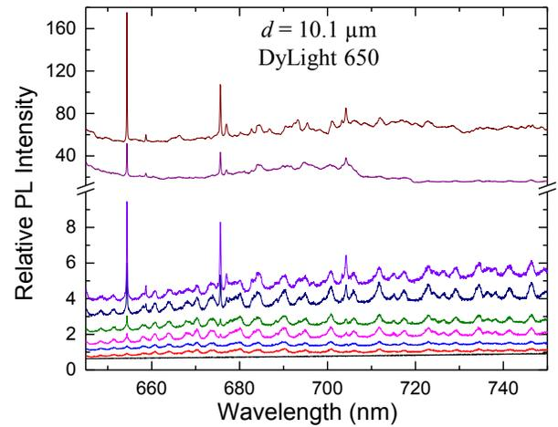
**Fig. 2.** Photoluminescence (PL) spectra for the optoplasmonic system in the 650-750 nm region. Nine spectral scans, recorded for  $\lambda = 632.8$  nm pump powers ranging from 24 nW to 2.0 mW, are given.
